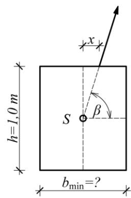
The position of the fixing point depends only on the tangent of the tent at the fixing point, so:  $x_b = x_a = 0,073 \text{ m}$
