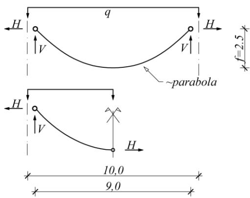
Loading zone:  $A = 10 \cdot 10,0 \text{ m}$ . Load-bearing zone:  $4,0 \cdot 9,0 \text{ m}$
