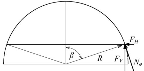
The horizontal force is balanced by the curved geometry of the foundation. The internal normal force in the circular foundation: (Barlow's formula)
