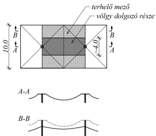
Static model – parabola form is assumed
