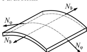
$$p_{\text{E,d}} = \frac{N_{\varphi}}{R_{\varphi}} \rightarrow N_{\varphi} = p_{\text{E,d}} \cdot R_{\varphi} = 2,6 \cdot 11,21 = 28,9 \text{ kN/m}$$
