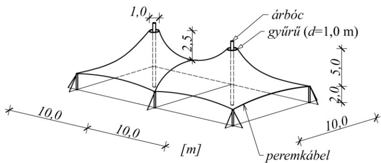
Pre-tensioning: ~1,0 kN/m applied at the edge cables.
