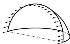
(the membrane force  $N_9$  equals to the membrane force  $N_9$  calculated at the elliptic part! see: 3D sketch)
