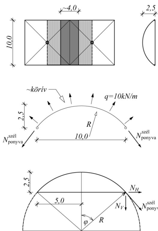
Suction: direction of the opposite curvature (to the previous one) is acting (similar to lightweight roofs)
