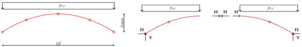
Analysis of existing geometry: data as in the exercise on the flat arch ( $p_{ed}=25\text{kN/m}$ ,  $l=1,5\text{ m}$ ,  $h=25\text{ cm}$ ), however now we would like to know the value of  $t_{min}$ ! **The support reaction forces are assumed to be the given (H (28 kN), V (18,75 kN), same as for the flat arch)!**
