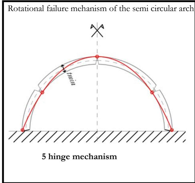
Structural model based on the five-hinge mechanism ( thrust line in red, hinges indicated).
