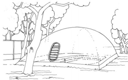
**Pneumatic tubes:** behaves similarly to the inner tire of a bicycle. Cylindrical or sphere like structures are typical. These pressurized inflated elements are shaped to carry load in a traditional manner. Mechanical equipment is also required to maintain overpressure in the structural elements, but as volume of the escaping air is smaller, so the required energy to obtain the overpressure is also smaller than in the case of one-layer air supported structures.
