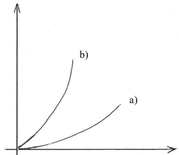
The force-displacement diagram of a cable a) without and b) with prestress.
