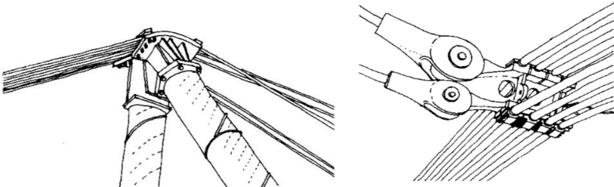
*Cables connected to other load-bearing components.*
