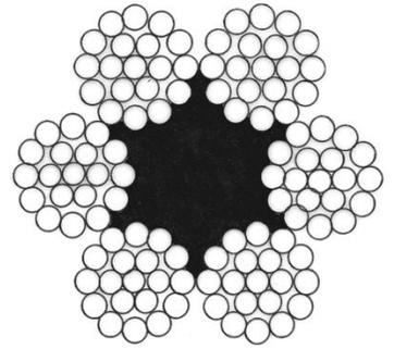
The metal wires are usually made of high-strength steel with a strength around  $1000 - 2000 \text{ N/mm}^2$ . Since the cable is not completely made of steel, its tensile strength is usually around  $500 - 1000 \text{ N/mm}^2$ .
