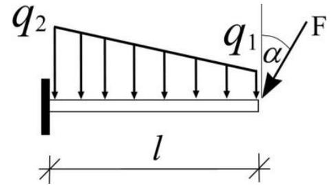
4. A cantilever with the length of  $l$  is loaded by a trapezoid distributed load and a skew concentrated load according to the figure.  $l=2$  m,  $a=30^\circ$ ,  $F=10$  kN,  $q_1=2$  kN/m and  $q_2=4$  kN/m.
