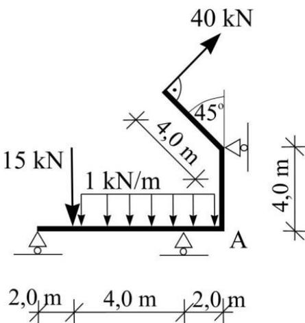
2. Given a beam with broken segments (see the figure on left).
