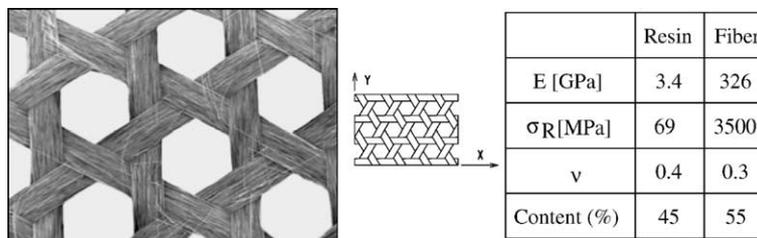
Fig. 1. Textiles layout and properties of materials.
