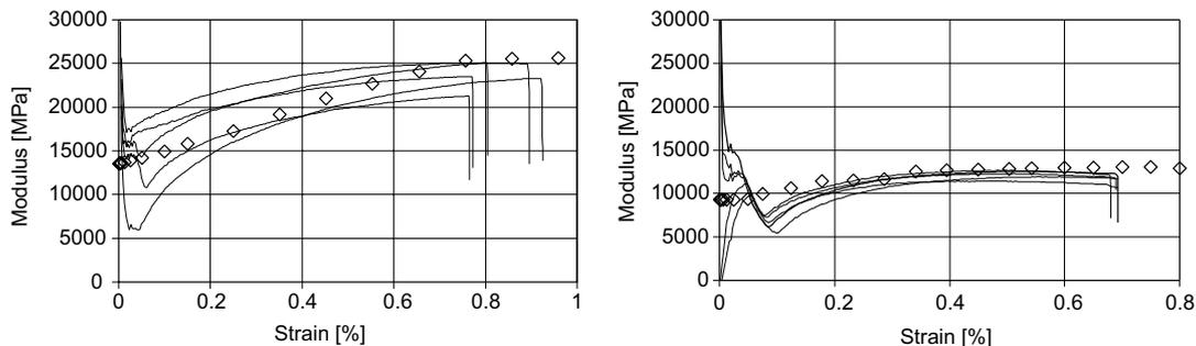
Fig. 6. Material stress–strain curve and results of nonlinear analysis (◇ numerical; — experimental).
