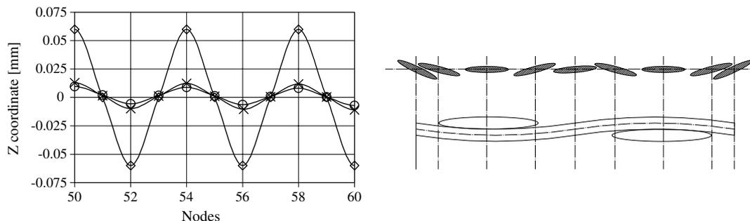
Fig. 7. Nodal position variation along yarn axis (–◇– undeformed; –○– strain 1%; –×– strain 2%) and section rotation along yarn axis.
