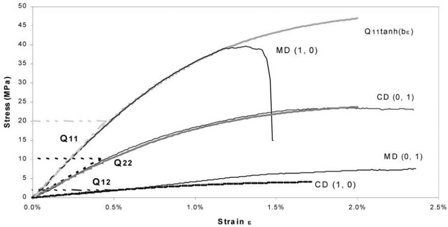
Fig. 8. Fitting of stress–strain curves for loading cases (1.0, 1.0) and (0.0, 1.0).
