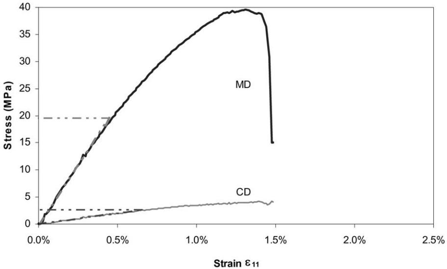
Fig. 4. Stress–strain curves case (1.0, 0.0); recall Table 1.
