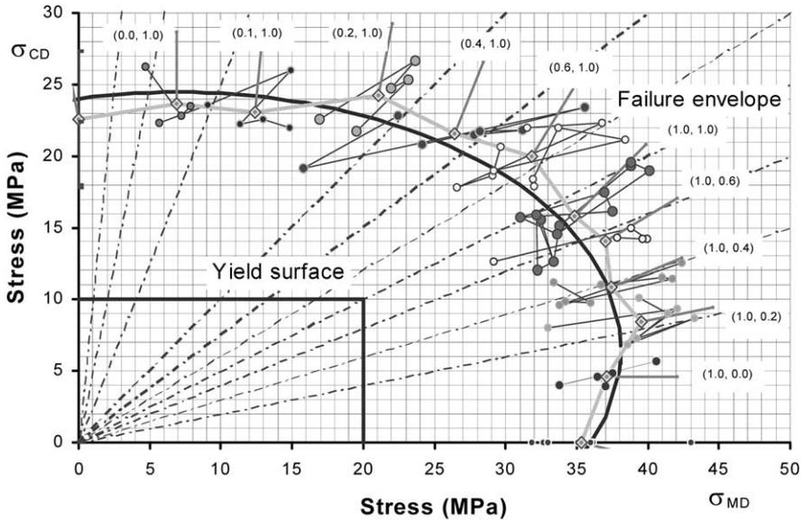
Fig. 7. Yield surface and random failure envelope of paper. Points of failure having the same loading designation are joined segments, and marked by the same color.
