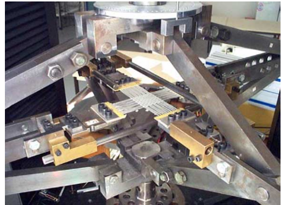
Fig. 3. Biaxial tensile device on cross shape specimens.
